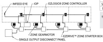
**EZLOGIC**\* **ZONE CONTROLLER**—Located in each zone (Retro-Reflective). NEMA 1, 2, IP 62. UL Approved.
