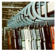
**Powered Over-N-Unders** utilize a standard Unibilt drive to move parts from load to unload. Powered Over-N-Unders are not restricted to straight loop designs. Horizontal turns and vertical curves can be incorporated to bypass aisles and other obstacles.
