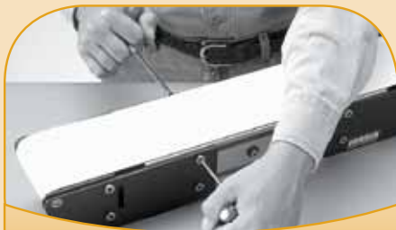
Rack and Pinion Belt Tensioning
